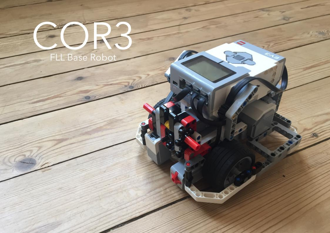
This Robot is designed for use in FLL and for teaching purposes. It is very easy to build new tools for and, most importantly, it can be built from a single MINDSTORMS EV3 education set.
